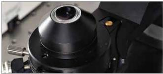
• Condensers - fully motorised focus Accepts both air and oil immersion condensers, including those required for DIC contrasting. Motorised for optimal Koehler illumination.
