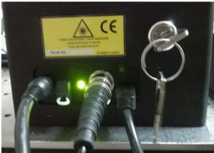
Figure A: Laser interlock is connected, and the laser key has been inserted and turned clockwise to enable emission. Green light indicates emission enabled.
