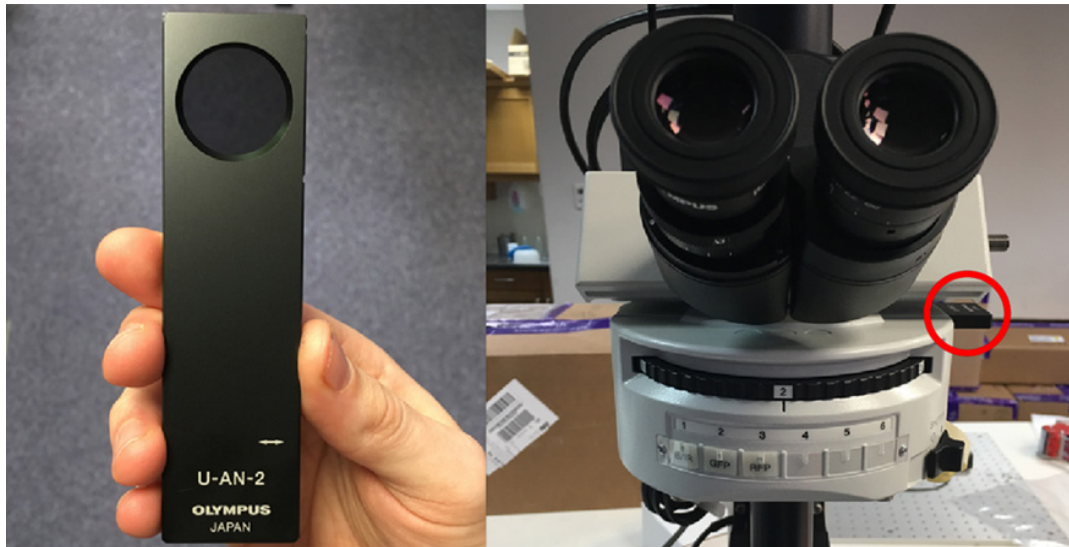
The image on the left is a U-AN analyser, and the image on the right shows the U-AN analyser inserted into a fluorescent turret on the SliceScope.
